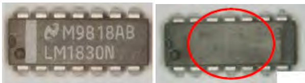
Figure 3-6: Marking confirmation with acetone.
