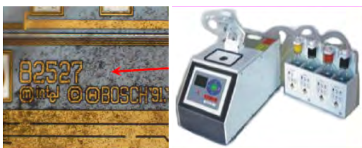
Figure 3-7. Device name can be checked after decapsulation.
