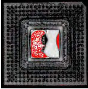
Figure 3-8: C-scan of BGA with severe delamination
