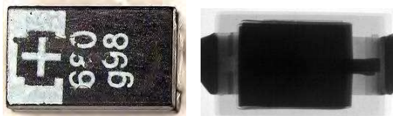
Figure 3-5: One can see the ink mark on the outside of the package but X-ray imaging reveals reverse polarity.
